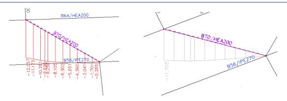
No the maximal relative deformation is taken as the deformation minus the deformation of the fixed node.
