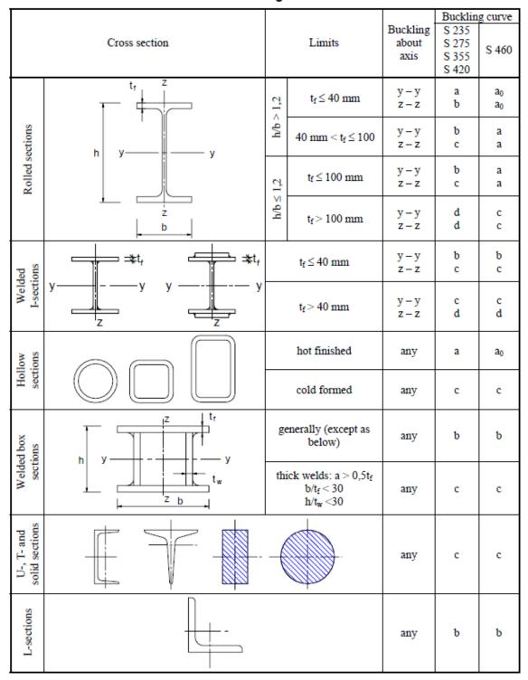
Table 6.2: Selection of buckling curve for a cross-section
