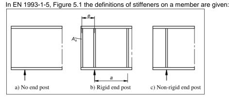
Those stiffeners will influence the total length for shear buckling. Also in SCIA Engineer those stiffeners can be inputted on a beam and will only have influence on the shear buckling check.
