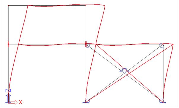
Calculation of  $\eta_{init}$   $\rightarrow$  To be filled in as 'max. deformation' (see 'Nonlinear combinations' window)
