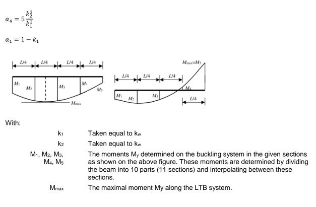
This method is only supported in case both k and  $k_w$  equal 0.50 or 1.00.
