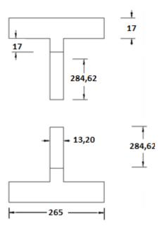
In this calculation the roundings at the corners between the flanges and the web are not taken into account. Therefore the result in SCIA Engineer will be a bit higher:
