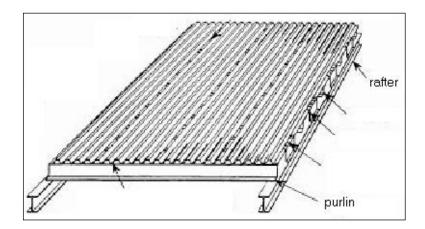
A sheeting can be inputted in SCIA Engineer via "Steel -> Beams -> Member Check data -> Sheeting":
