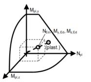
The yield surface is generated for the given section and the intersection of the actual forces is determined with this surface.
