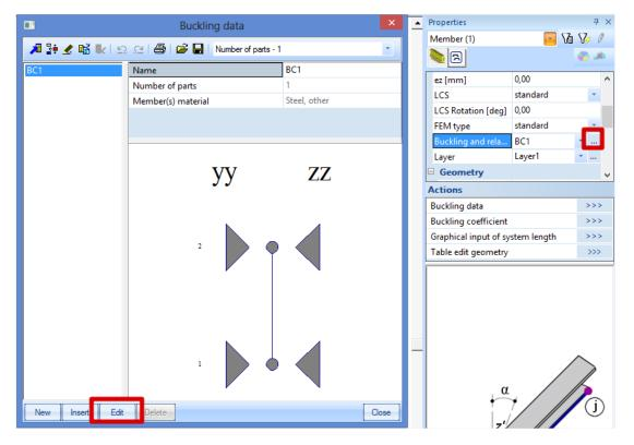
Click on Edit button and go to Buckling data tab, here you can modify the values for k and kw:
