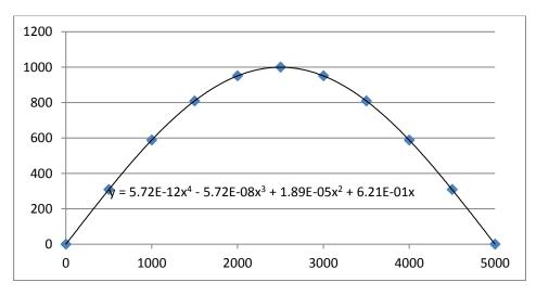
A polynomial has the advantage that the second derivative can easily be calculated.
