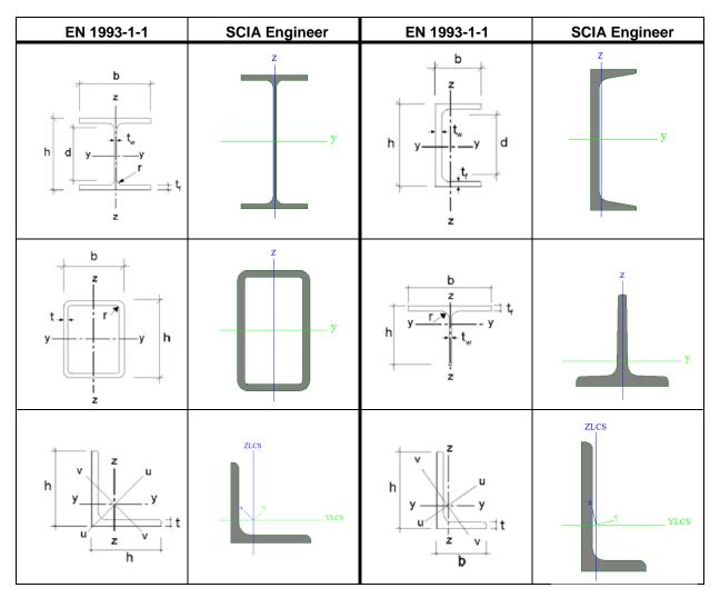
In the steel code check, the strong axis will always be considered as the y-y axis. So when inputting a profile in which the local y-axis does not corresponds with the strong axis, the axes are switched in the steel code check and SCIA Engineer will give a message about the axes.
