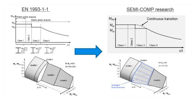
If the classification results in a class 4 profile, the effective cross section will be calculated according to EN 1993-1-5.
