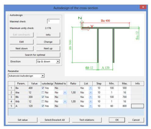
So the thicknesses thb and tha are not autodesigned. All other options can be adapted by SCIA Engineer. When clicking on "Search for an optimal", the following profile is suggested by SCIA Engineer:
