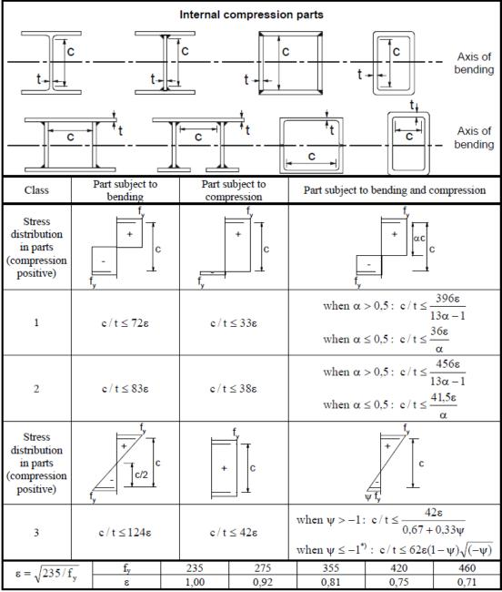
\*)  $\psi \leq$  -1 applies where either the compression stress  $\sigma \leq f_y$  or the tensile strain  $\epsilon_y > f_y/E$
