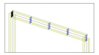
Those stiffeners can be inputted via "Steel -> Beams -> Member check data -> Stiffeners".
