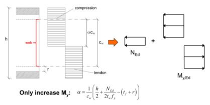
Within this formula the N<sub>Ed</sub> is taken as positive for compression and negative for tension.
