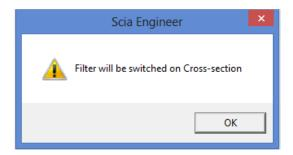
And in the properties window the option for "Filter" has been changed into "Cross-section". Now choose here for the profile IPE 140 and click again on "Refresh" and afterwards on "Autodesign".
