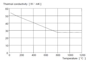
For  $20^{\circ}C \le \theta_a < 800^{\circ}C$ :  $\lambda_a = 54 - 3,33 \ x \ 10^{-2} \ \theta_a \ W/mK$
