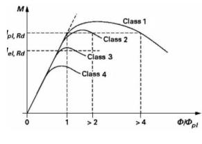
This classification depends on the proportions of each of its compression elements. For each intermediary section, the classification is determined and the related section check is performed. The classification can change for each intermediary point.
