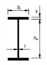
If the slenderness is higher than the minimum one, the shear buckling check is executed following EN 1993-1-5, formula (5.10) (this is a check on the shear force) and formula (7.1) (which is the check on the interaction between shear force, bending moment and axial force). Both formulas are checked in SCIA Engineer.
