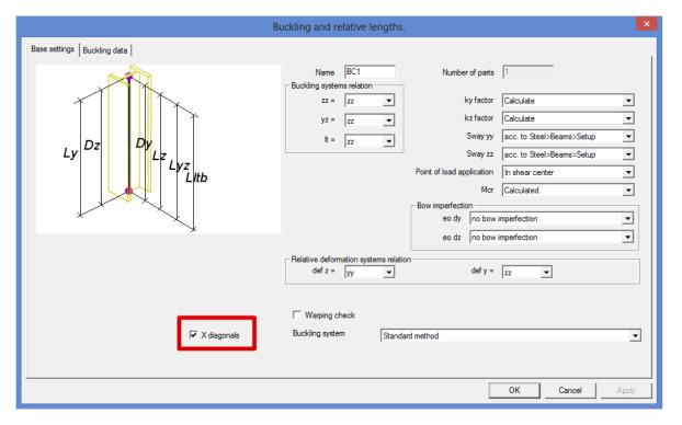
If this option is used, SCIA Engineer will use the method from the DIN to calculate the buckling factors for the diagonals.
