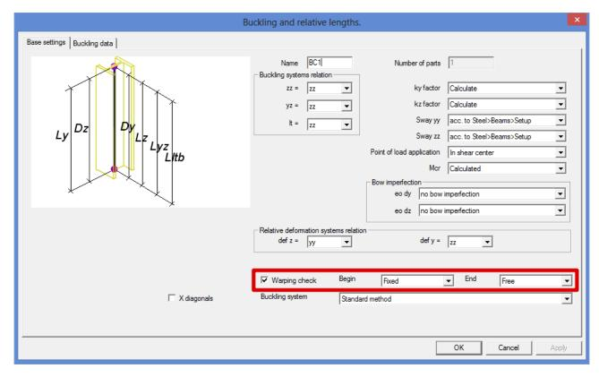
The check box **Warping check** should be activated and for the beginning and end of the beam, the user should indicate if this end is Fixed or Free for warping.
