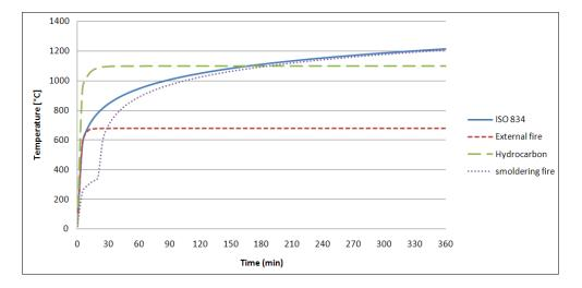
Standard temperature-time curve:  $\Theta_g = 20 + 345 \log_{10}(8 t + 1)$  [°C]  $\alpha_c = 25 \text{ W/m}^2 \text{K}$
