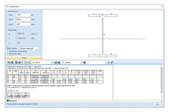
In the cross-section properties, the user can choose the plastic analysis method. However, this is only informative and this choice is not decisive. The method that will be used to perform the steel code check can be chosen in the **Steel setup** window:
