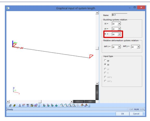
The reference length can be overruled by another value using LTB restraints. These restraints make it possible to define separate conditions for bottom and top flange.
