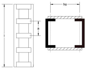
Example – manual calculation of a battened compression member
