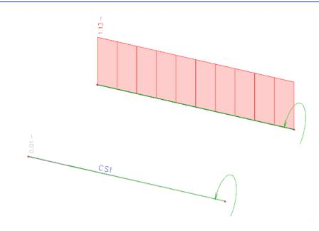
The difference in the results is in the torsion check. For the first beam no torsion check can be executed, since no results for torsional stiffness's can be found.
