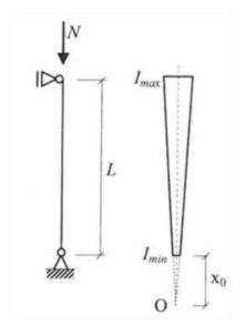
Hirt and Crisinel Ref[xx], present expressions for the elastic critical load of axially loaded non-prismatic members of double symmetric cross-sections (i.e. I sections formcode 1). Flexural buckling around the strong axis of the cross-sections occurs for:
