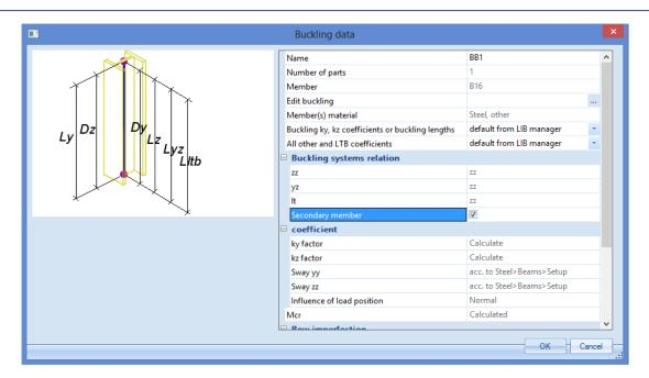
When looking now at member B13 and changing the Buckling and relative lengths back to "defaults" the member B16 will not be included in the system lengths:
