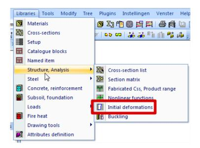
Since this example is made in a 2D-environment, one initial deformation for the x-direction is sufficient. If the project was made in a 3D-environment, it would be needed to create two initial deformations (one in x-direction and one in y-direction).
