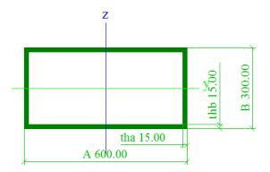
This beam is only loaded by a line load in the z-direction, resulting in a moment My and a shear force Vz on the beam.
